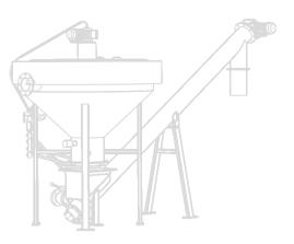
A classifier installed in Hagenbrunn, Austria. The unit was entirely workshop-assembled in stainless steel and has a capacity of 11 l/s. After washing, the collected sand has an organic content of less than 3% by volume. The building is odour-free.
